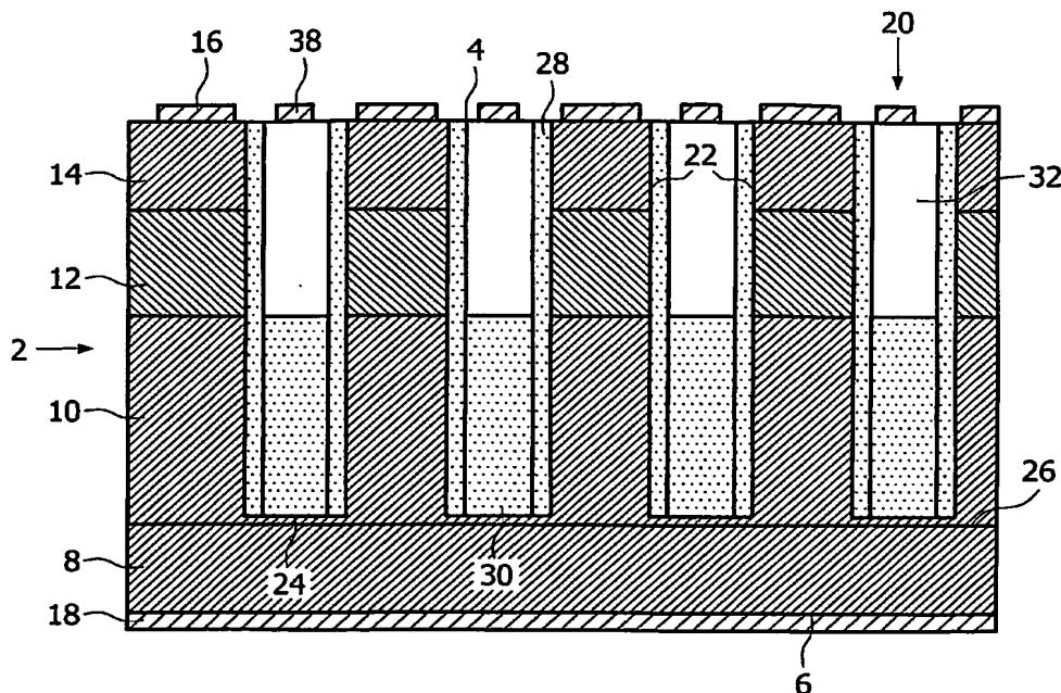
(57) Abstract: The invention relates to a trench MOSFET with drain (8), drift region (10) body (12) and source (14). In order to improve the figure of merit for use of the MOSFET as control and sync FETs, the trench (20) is partially filled with dielectric (24) adjacent to the drift region (10) and a graded doping profile is used in the drift region (10).
